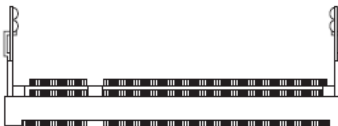
DDR2 SO-DIMM Slot 200-pin, 1.8V
